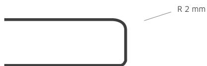
The bigger the radius the better it will withstand impacts but it will also show more of the base colour of the slab. In areas with a high risk of impact (sinks for example) a 2 mm Radius Edge is recommended; it is the best option between aesthetics and durability. The edges portrayed here can also be applied on mitered edges.
